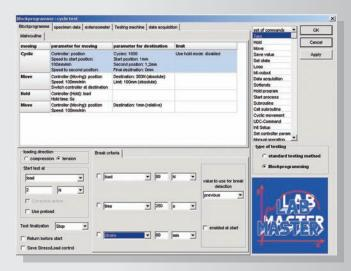
The block programme offers a sequential list of movement, hold and control commands. They allow for cyclical movements, relaxations and creep tests, e.g. for fracture mechanics or component testing. The commands are parameterised in windows, which doesn't require any programming skills.
