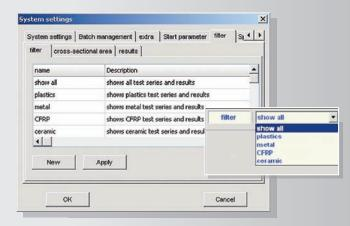
LabMaster content can also be tagged and filtered for a more clearly arranged organisation. The displayed data can then be reduced by selecting only those tagged with a specific filter. Filter tags can be created by the user and explained with descriptions.
