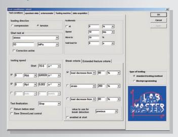
All of the settings relevant to the test are done in this menu. This includes e.g. test speed, switch points and breakage identification criteria. A standard test is defined with few settings. The specimen geometries for routine testing can be entered or imported from external sources before the test starts. Due to the structure of the database there are no restrictions to the naming and storage of the measuring results.
