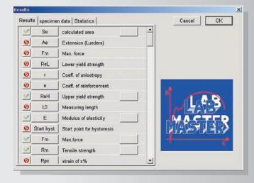
The post calculation function that is included in the software allows for a convenient subsequent change of test conditions, e.g. cross section surface or breakage identification criteria.
