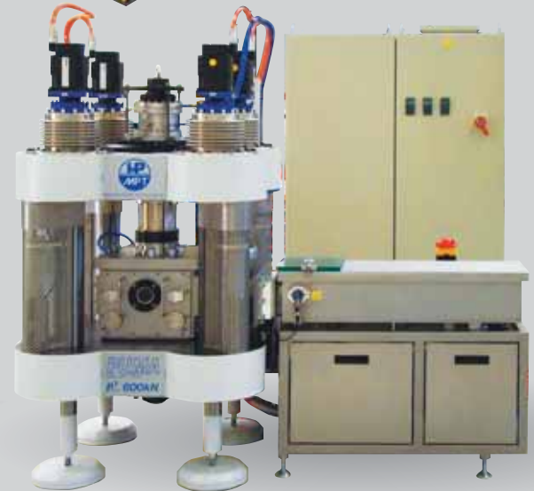
INSPEKT P.U.MA 600 kN This metal forming test equipment is used for research purposes to characterise micro deformation processes. Four separately controllable drives ensure an exact plane parallel introduction of the force. The deformation processes takes part in a vacuum with temperatures of up to 1200 °C.
