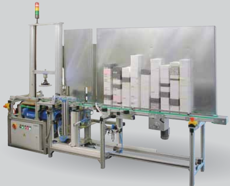
Fully automatic testing system for foam material. This system is based on an INSPEKT table 5 kN machine for pressure and bending tests and a specimen measuring station. A pneumatic linear feeding system guarantees a high specimen throughput.
