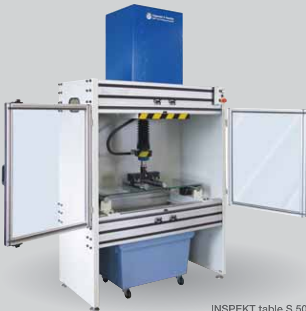
INSPEKT table S 50 kN Universal testing machine for safety glass in the building industry and in shipbuilding. The machine has been designed to carry out pressure tests as well as 3 and 4-point tests.
